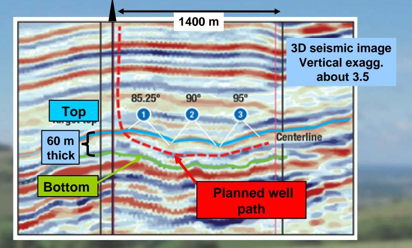
This is an example from the Woodford Shale, USA, of guiding the horizontal drilling, the real-time position of which is overlain on a vertical slice of a 3D seismic image, the 'backdrop'. This is simple geology, unlike the UK, in which the dip (slope) of the target layer is within 5° of the horizontal, as measured by the three average figures shown in the centre of the image (90 ° = horizontal). Other examples can be found in the paper by Mottahedeh (2005).
