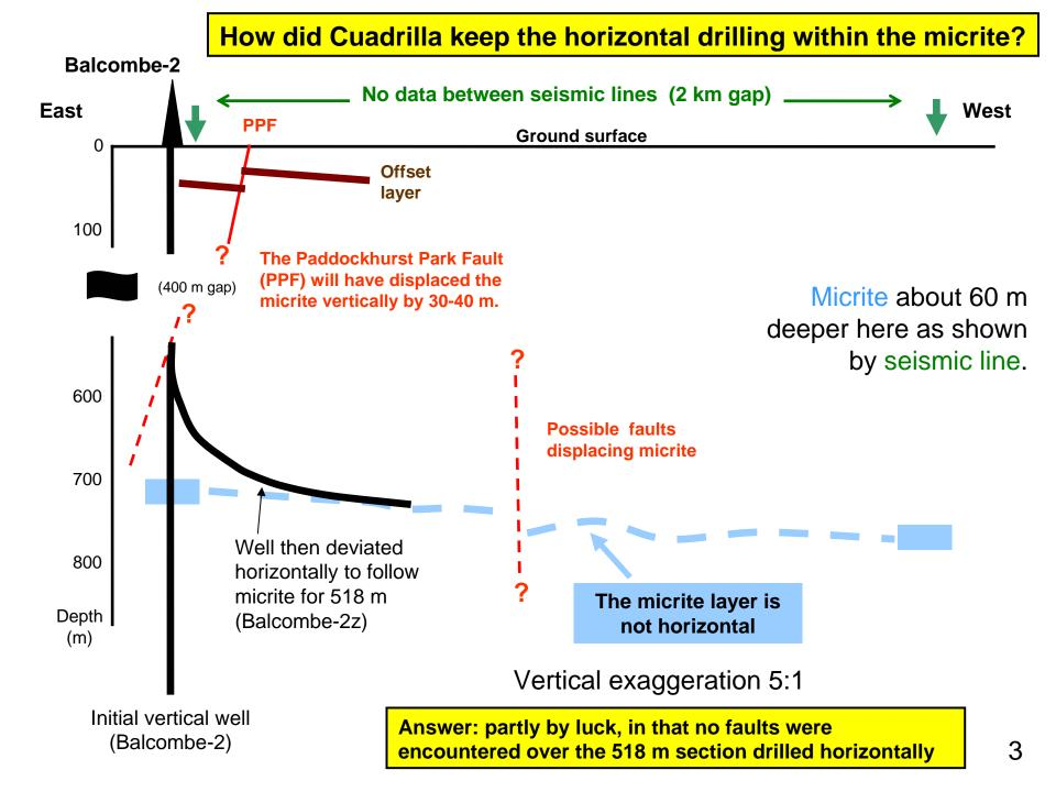
So Cuadrilla was steering 'blind', except that the drill-bit could sense the roof and floor of the limestone layer and keep to the middle of the layer.
