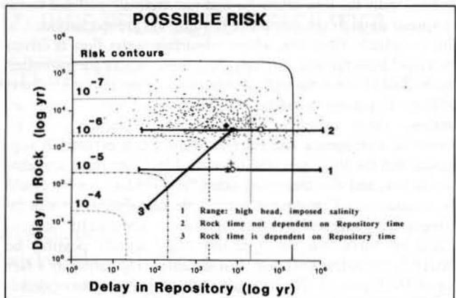
Figure 3 The overall modelled risk from a repository, adapted by H Wallace from report Nirex 95. Contours show risk of 10<sup>-6</sup>, 10<sup>-5</sup> etc. If BVG is modelled as increased permeability, so both x-axis (time in repository) and y-axis (time in geosphere) values decrease. Consequently the overall risk modelled by Nirex (square) is likely to be too low, and the true risk moves along line 3.
